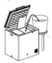
(4) Insert the suction hole of the water suction device into a water container and insert the water outlet into the water tank. Continuously squeeze the air cell of the water suction device with hands. In this way, the water flows from the container to the water thank. Stop to squeeze the air cell when the water begins to flow and the water will automatically flows into the water tank.
